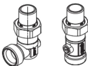
This single connection fitting is for shut-off, not for reduction.
