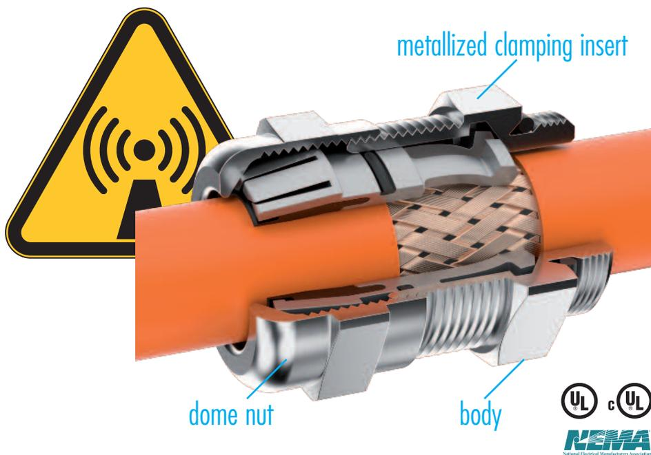
The metallized clamping insert ensures a secure 360° contact to the shielding braid and thus permanent EMC protection even in dynamic applications.
